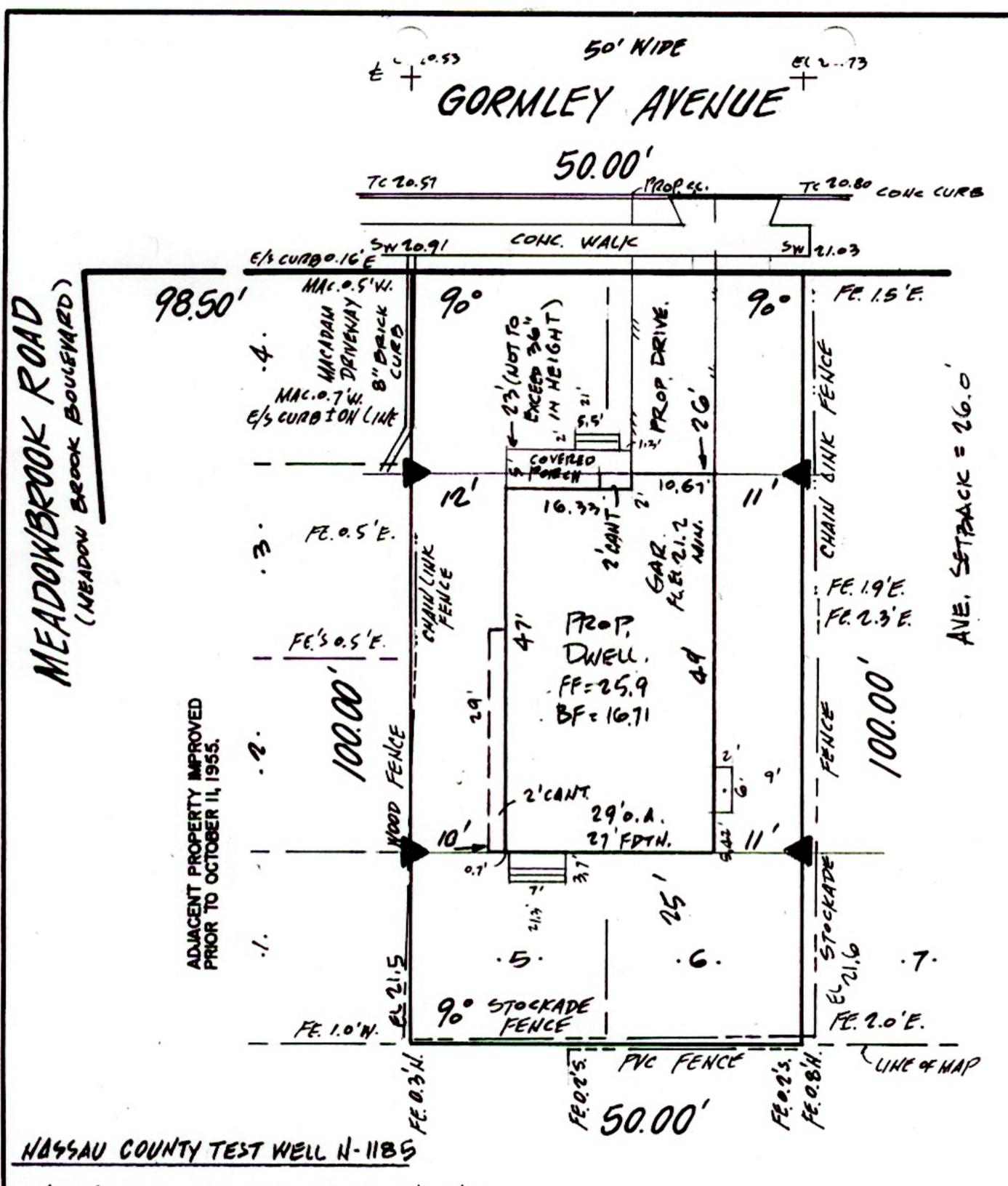
MAX. GROUND WATER EL. 15.21 5/25/56 + SAFETY FACTOR 1.5 MIN, BAYEMENT FLOOR GL. 16.71
